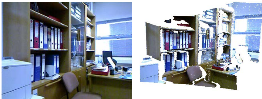
Figure 1.6: Example of one frame data from the ViDRILO Dataset. Color image on the left and point cloud on the right.
